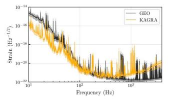
**Figure 1**: (The left panel of Fig. 1 from our publication) Plot showing the typical sensitivity of KAGRA (yellow) and GEO (black) during the joint observing period. The vertical axis gives the average strain noise in the detectors, which is a measure of how much the mirrors typically move as a function of frequency (horizontal axis). The solid curves show the mean sensitivity for each frequency bin and the shaded regions show the 5th and 95th percentile over the period.
